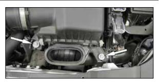
5. Remove the two bolts that secure the air filter housing to the core support and then remove the air filter housing from the vehicle.
