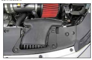
16. Reinstall the fresh air intake duct and secure with the factory push pins.
