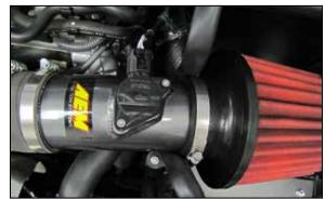
15. Reconnect the mass air sensor electrical connection.
