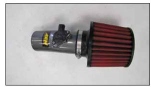
13. Install the AEM® air filter onto the intake tube and secure with the provided hose clamp.
