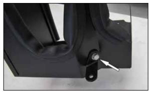
8. Install the provided bracket (064355) onto the heat shield using the provided hardware.
