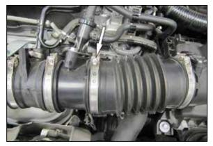
3. Loosen the hose that secures the intake hose to the turbo inlet pipe.
