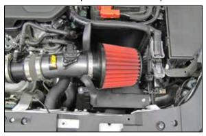
14. Install the intake tube assembly into the coupler hose at the turbo inlet pipe, adjust the assembly for best fit and then secure with the provided hose clamp.
