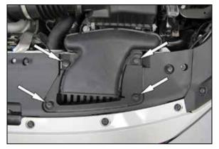
4. Remove the push pins that secure the fresh air duct and then remove the fresh air duct from the vehicle.
