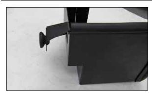
7. Remove the mounting grommet from the factory air filter housing and install it into the AEM® heat shield as shown.
