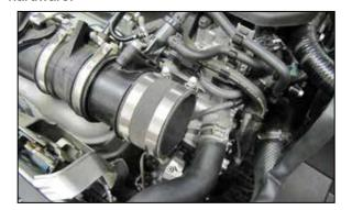
11. Install the provided coupling hose (08711) onto the turbo inlet pipe and secure with the provided hardware.
