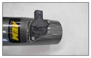
12. Remove the mass air sensor from the factory air filter housing and then install it into the AEM® intake tube and secure with the provided hardware.
